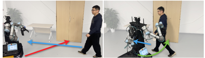
(a) Motion-level. Left: The human’s movement interferes with the robot’s approach to the door. Right: The robot must dynamically adjust its movement to avoid colliding with the human.
